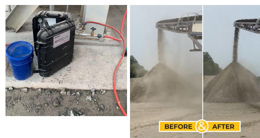
Figure 4. Using a dust suppression system (left) and results of implementation (right) (source: https://benetechglobal.com/products/minipak-dust-suppression-system/ )
